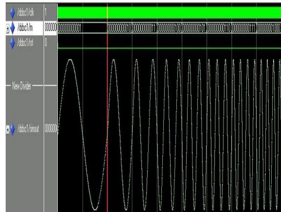
**Figure 9. Simulation Results of DDS in MODELSIM**
