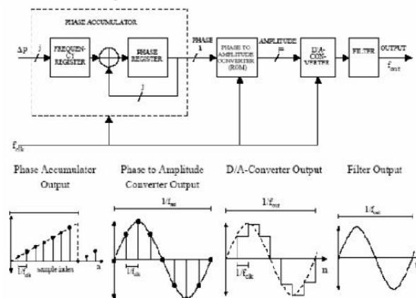
Figure 6. DDS Block Diagram with DAC and Filter
