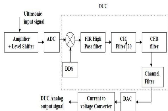
Figure 1. Digital Up Converter Block Diagram
