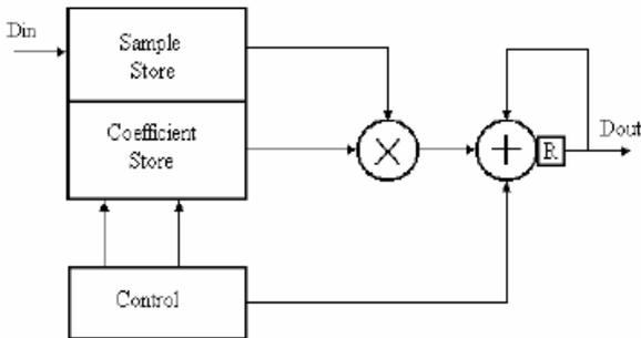
**Figure 7. Simplified Block diagram of MAC**
