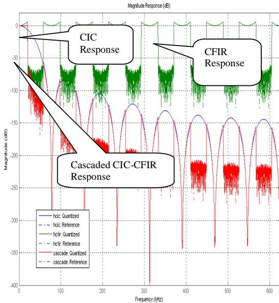
**Figure 8. Working of the CIC-CFIR Filter and its Combined Response in MATLAB**
