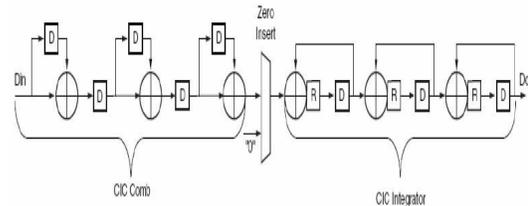
**Figure 2. CIC Filter Structure Block Diagram**
