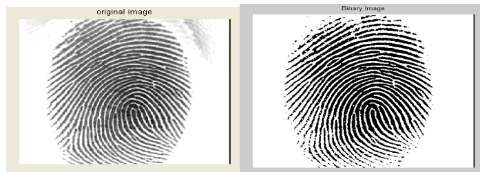
Figure 2. Original Fingerprint image (left), Fingerprint image after adaptive binarization (right)
